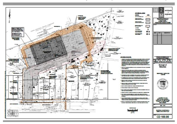
Drawing included in demolition bid for 'reference only', as it is an extract from the separate bid set. As such, the limit-of-disturbance language for the existing building demo work is listed as 'Not-in-Contract'.
