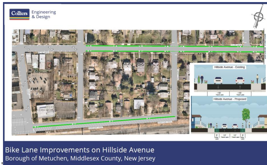
Figure 2: The Sixty (60) Percent Design by Colliers Engineering and Design shows the Hillside Avenue Bikeway Road Markings on Hillside Avenue, Station Place and Pennsylvania Avenue.
