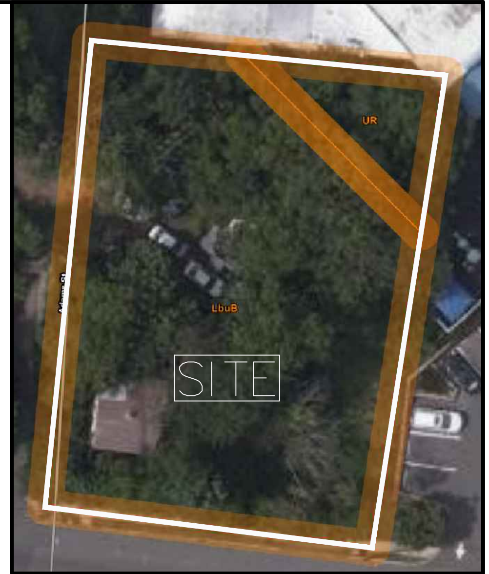
SOILS MAP SCALE: 1"=30' MAP SOURCED FROM USDA WEB SOIL SURVEY THE SITE IS MADE UP OF: LbuB (LANDSOWNE-URBAN LAND COMPLEX, 0 TO 6 PERCENT SLOPES) UR (URBAN LAND)
