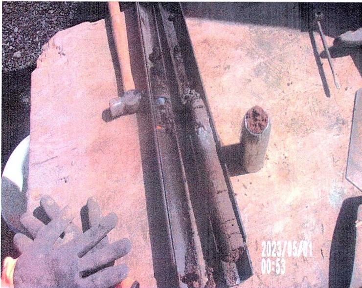
Sample recovery from split spoon samplers
