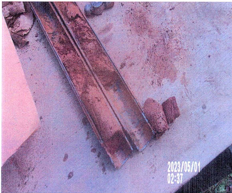
Sample recovery from split spoon samplers
