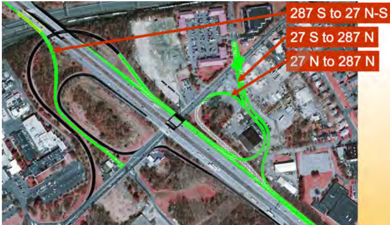
One of several options for proposed New Jersey State Route 27 & Interstate 287 interchange.
