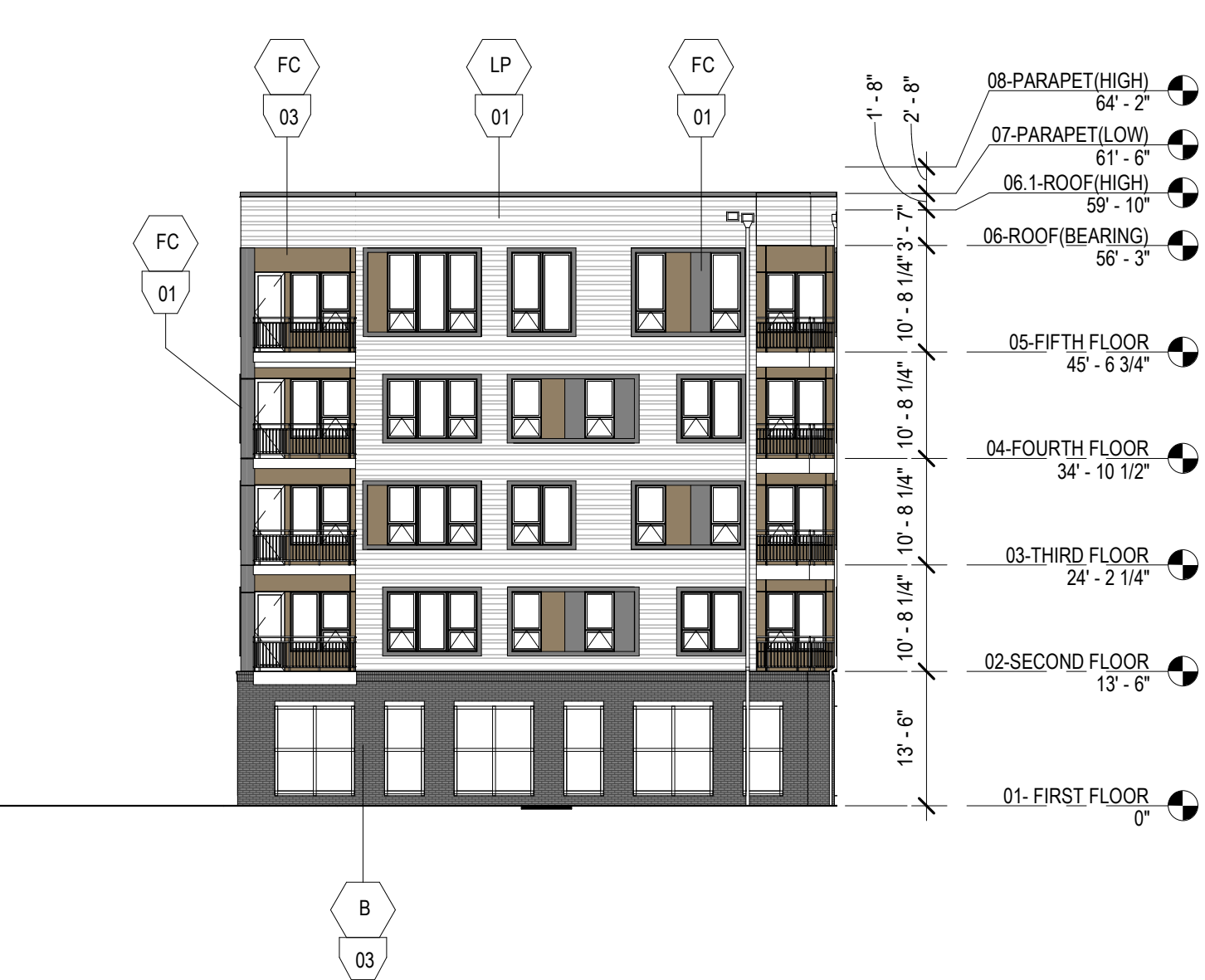
NORTH CORNER ELEVATION. 5 1/16" = 1'-0"
