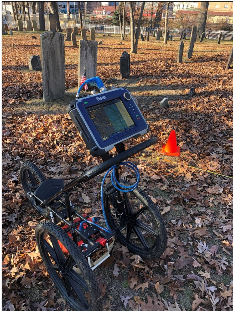
Plate 3. IUP GSSI SIR-4000 GPR system at Metuchen Colonial Cemetery.
